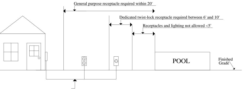
Branch circuit for permanent pools (those capable of being filled with over 42" of water) shall be pulled in electrical non-metallic tubing (pvc). Burial depth shall be a minimum of 18". Receptacles shall be GFCI protected.
